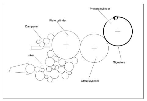
Ink is transferred to the plate cylinder by an inker and dampening solution by a dampener. The ink is transferred from the plate cylinder to the offset cylinder and only then is it printed onto the stock. It is easy to deduce that the printing dots (or pixels) are flattened during these transfer operations.
