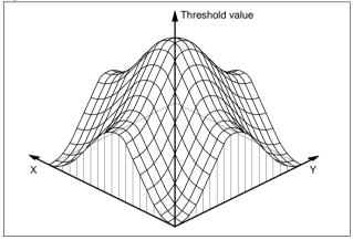
The various screen angles are created by converting the coordinates from the coordinates system of the recorder to the coordinates system of the dot matrix which is mainly rotated.
