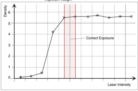
Gradation curve of a hard dot film with the correct exposure range:
