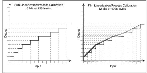
Calibration with 8 bit and 12 bit resolution:
