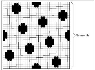
Diagram of a screen composed of screen tiles:
