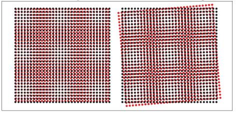
Moirés can occur not only in the overprint of screens which do not match but also between fine, even patterns in the original and the screen. For example, they can occur between the stripes of a shirt and the screen. This type of moiré can be avoided by using Diamond Screening which is described later on.
