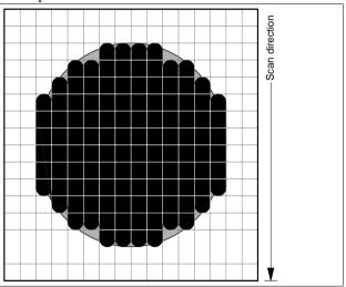
Diagram of a screen dot with double the resolution in fast scan direction (direction of rotation of laser mirror or drum) compared to slow scan direction (feed direction). The reproduction of the dot shape is considerably better. Size: 16x32 pixels:
