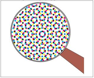
Colors C, M and K which provide more detail are spaced at an angle of 30°. The non-defining color Y must be positioned inbetween, spaced at an angle of 15°.
