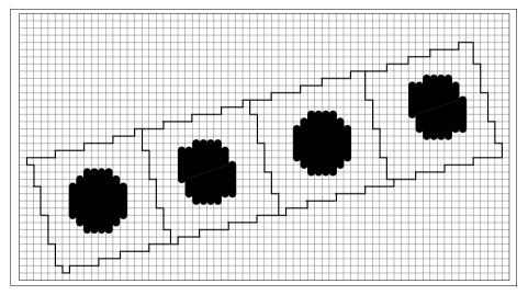
A dot matrix and not a screen tile forms the starting point for creating the screens. This matrix consists of 128 x 128 elements at present and the dot shape is filed as 12-bit gray values there.
