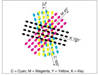
As can be seen in the table of relative screen frequencies below, yellow at  $0^{\circ}$  is somewhat finer than the other screens. This reduces yellow moiré which is possible with conventional screens. Refer to conventional screens (page 5–4).
