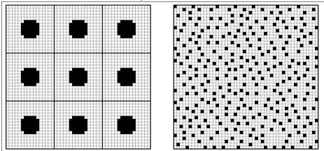
With Diamond Screening, it is possible for a print to have an almost photo-like quality. A sharpness in details is achieved which is not possible with any other system. Disturbing offset rosettes do not occur in this system. Your print comes closest to the quality of a color photo.
