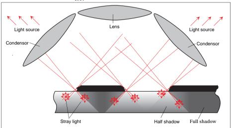
The diagram above shows how light reacts in the measuring head of a densitometer. The original is illuminated by condensor lenses attached to the side. The diffusely reflected light is projected onto a photo cell and measured by means of a central lens. Light mirrored on the surface does not fall onto the lens in this
