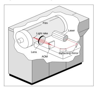
Diagram of an out-drum imagesetter:
