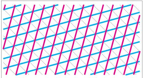
This screen overlaps with the black separation at 45°. If there are only minor deviations in the angle and screen frequency, a monotonous moiré or color shifts occur in many hues. This should not be dismissed too easily as not only quality inspectors with a trained eye (for example, in advertising agencies) see this and will quote really low prices.
