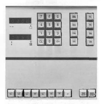
Fig. 2-18 Operator Control Panel of Electronics Cabinet
