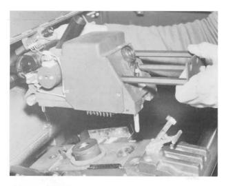
Fig. 5-5 Mounting or Demounting the Exposing Head for Halftone Separations
