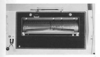
Fig. 2-11 Exposing Drum with Register Pins and Vacuum Channels, Viewed through the Front Panel with the Cassette Removed
