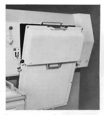
Fig. 5-7 Loosely Inserted Cassette
