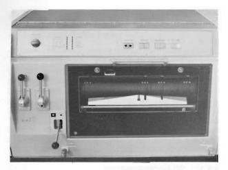
Fig. 3-8 Operator Control Panel above the Front Panel
