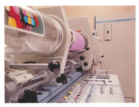
Salient features of this scanner are a clear operating sequence, short runthrough times, low material consumption, extensive correction possibilities and supremely versatile applications. Faster setting-up is particularly important. Controls and indicating signals are clearly laid out in functional groups. Faster setting up becomes possible by entering setting parameters via a functional keyboard and automatic micro-computer-controlled execution.
