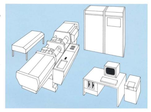
The Chromacom system\* uses the high-performance Chromagraph DC 350 S scanner. In its scope this is identical with the self-contained Chromagraph DC 350, but uses a modified system-compatible drive. The scanning and recording system includes, beyond the Chromagraph DC 350 S the process computer, data display terminal, two floppy disc drives and a 300 MB magnetic disc drive.
