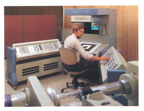
The Chromaskop is a system module that shows the anticipated printed result on a colour video screen while you actually set up the colour computer. The colour monitor screen directly shows the effect of every tone and colour correction control setting, without recording any film or going to the extent of pulling proofs. Hence you have all the advantages of previsualization without expenditure of materials or time.
