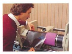
A separate mask drum facilitates image combinations, can introduce geometric patterns and lettering and permits partial image correction. That way it is possible to alter the colour in selected image areas or to modify the detail and contrast in different image
