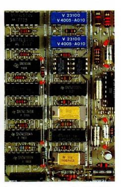
For axial scale changes the scanning and recording heads advance at different rates. The digital electronic system controls circumferential scale changes: While the drum rotates, the image signals of a scan line are digitised and fed to an intermediate memory. A fraction of a second later these signals pass to the recording optics with a compressed or expanded time scale.
