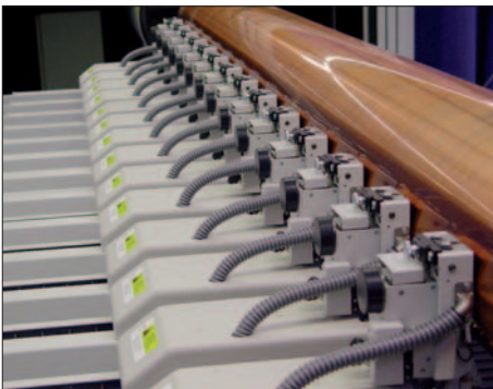
Top precision: Automatic axial and radial positioning of engraving supports.
