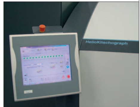
Simple to use: A touchscreen also allows the K6 to be operated manually if required.
