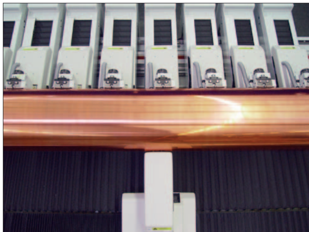
AutoSpacer precision for "Family mode": CellGuard controls the exact spacing of the stylus tips.
